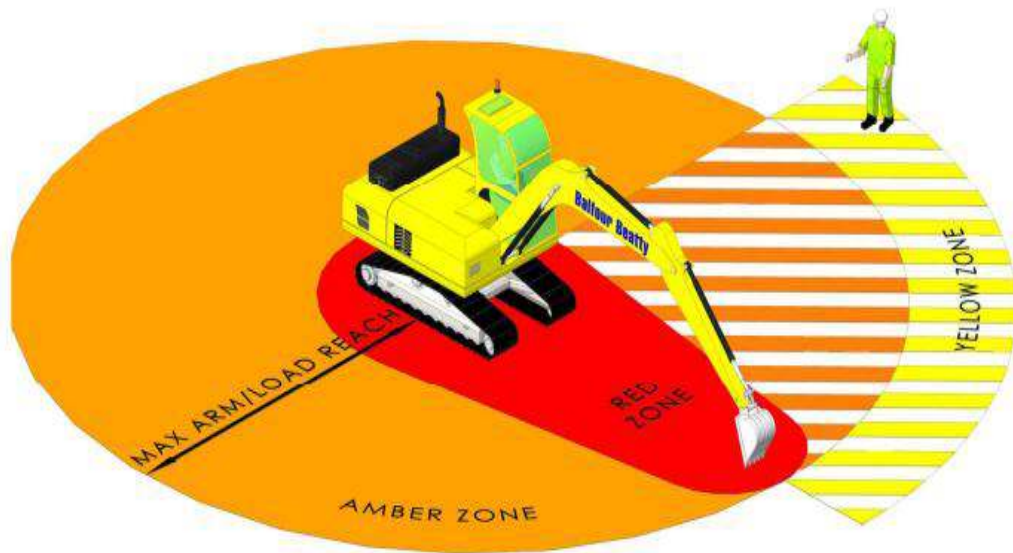
Gambar 6.17 Zona Keselamatan Bucket Excavator
